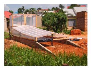
Figure 2: Solar dryer of Green Heat Uganda Ltd.
