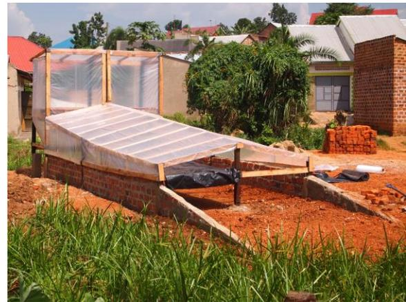
Figure 2: Solar dryer of Green Heat Uganda Ltd.
