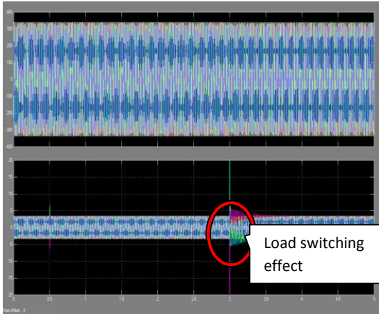
Figure 7: load voltage and current parameters
